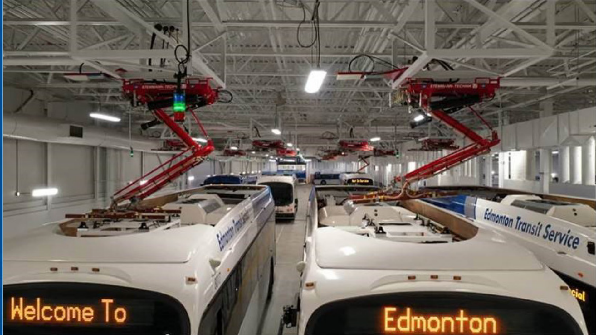
Edmonton Transit Service (ETS) battery electric buses charging by overhead pantograph charger.
