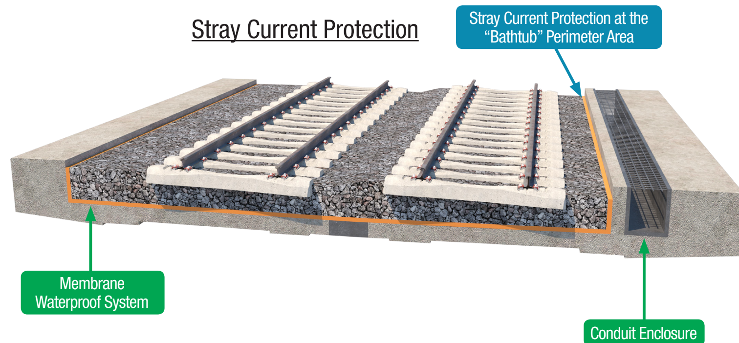
Figure A5.2.1-13: GLP has included stray current protection as part of our corrosion control techniques to reduce impacts from induced currents caused by the GLX traction power system that could lead to corrosion of nearby utility and systems that are susceptible to stray current.
