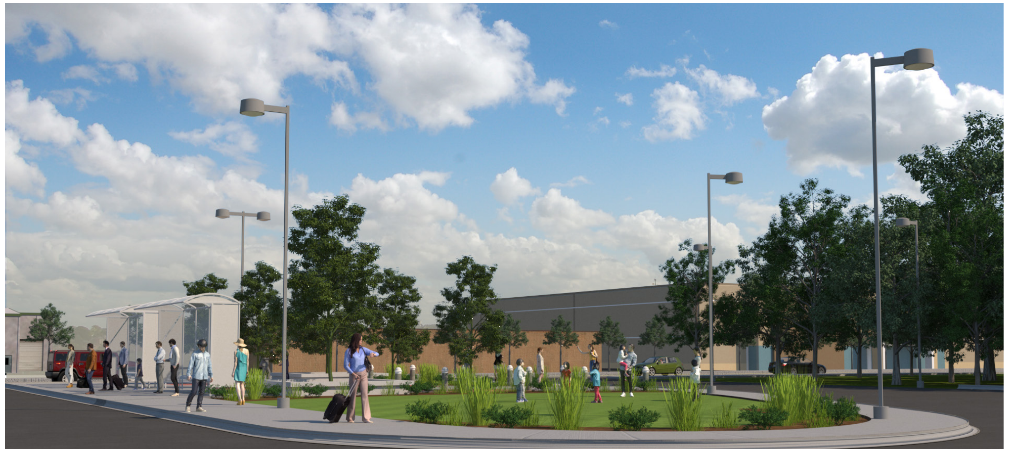
Figure A5.2.3-6: Low plantings do not block passengers’ views across the station, nor do they allow anyone to hide behind them. This is an example of Natural Access Control and is most successful with a maintenance plan to manage the height of the plantings.
