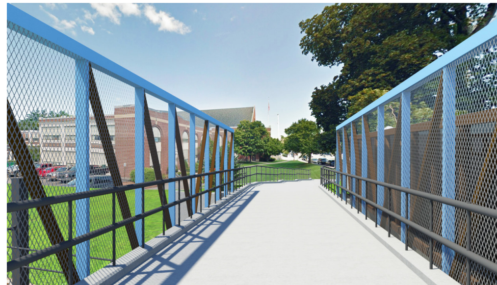
Proposed College Avenue Pedestrian Bridge. The above graphics show one possible prefabricated truss suitable for this location.
