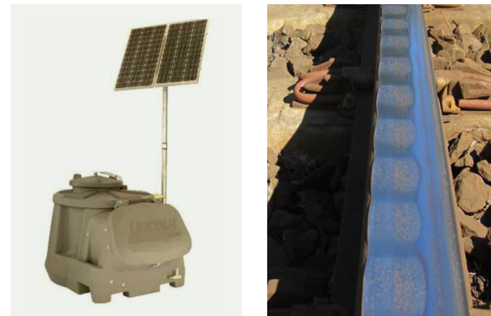
Figure 4.1-10 Rail corrugation preventions. A solar-powered wayside rail lubrication system (left) helps to combat rail corrugation (right).
